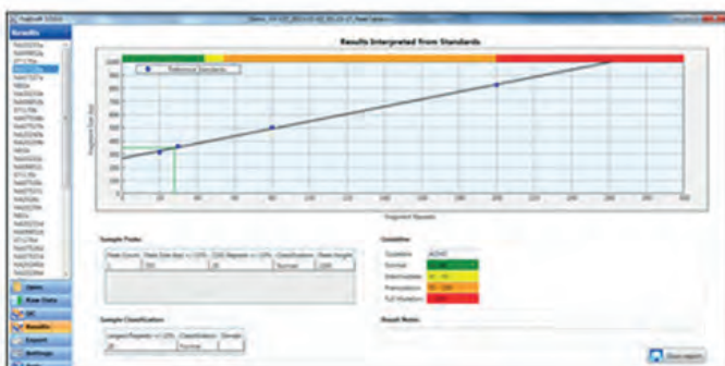
Microfluidic capillary electrophoresis analysis of a Coriell female normal sample (NA07538), and a Coriell male Fragile X sample (NA06852) with >200 repeats, together with the FraXsoft result interpretation and classification.
